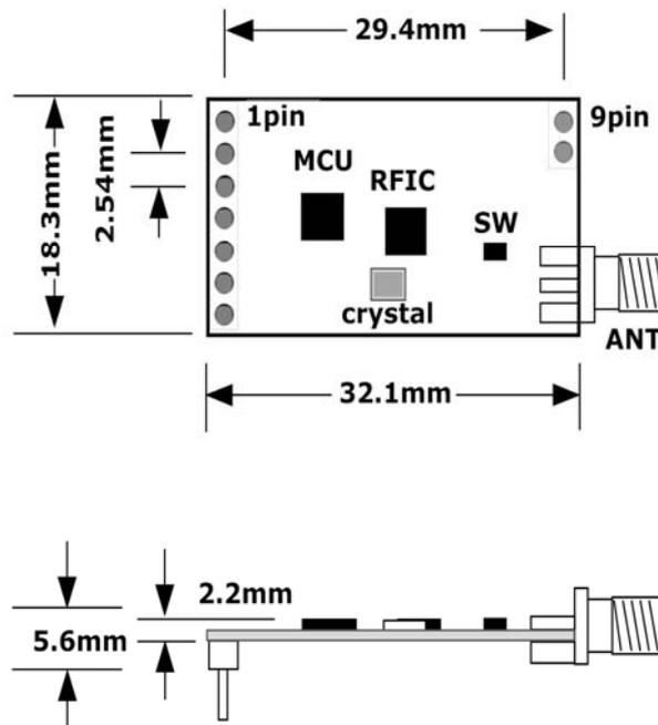
**Figure 6: Mechanical Dimension**
